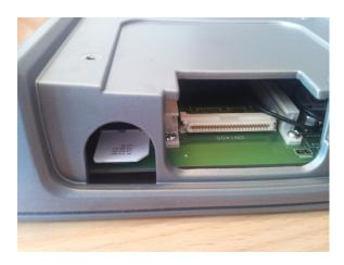
• Install top cover to prevent dust or other unwanted particles from entering the Airlink GX400.
